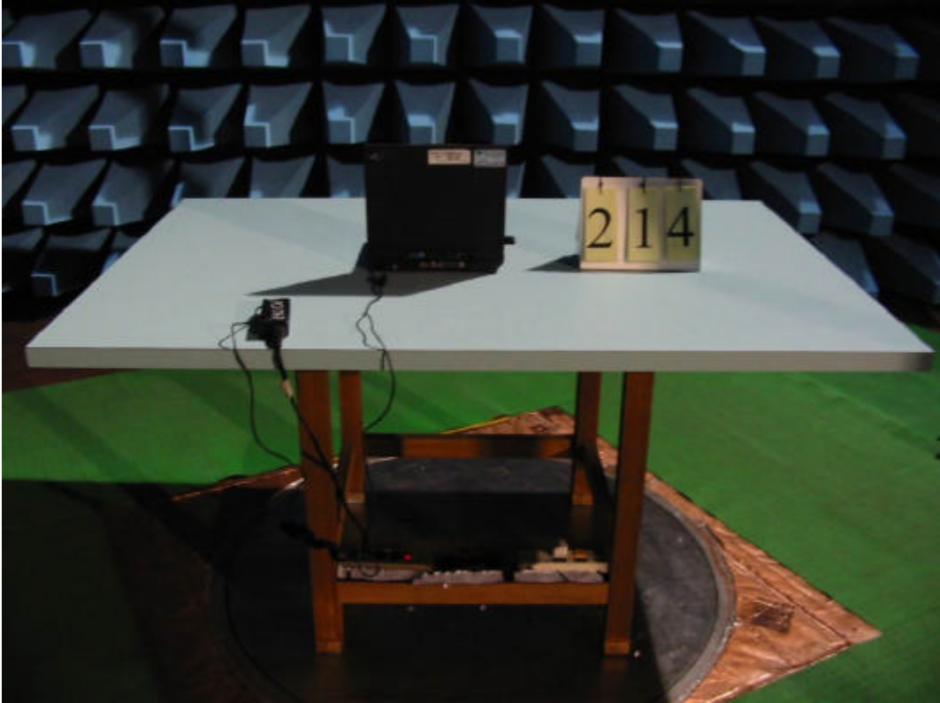
Rear View of the Test Configuration of Intentional
